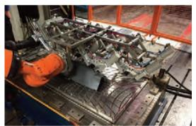
High grade SMC based material being placed in to an Aqua-floor shower deck mould using the UK's most technically advanced robotic SMC
