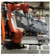
A freshly moulded Aqua-floor Shower Deck ready to be removed from its mould.
